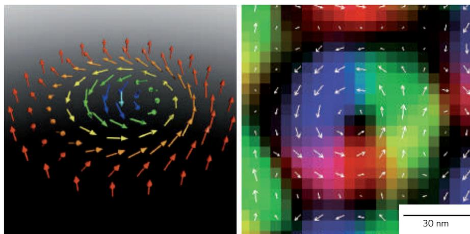
**Figure 1** | Skyrmions on the surface of  $\text{Fe}_{0.5}\text{Co}_{0.5}\text{Si}$ . Left, schematic of spin configuration in a skyrmion. Right, the colour map and the white arrows represent the magnetization direction at each point. The formation of these magnetic structures is one of the many phenomena occurring in strongly correlated materials. (Adapted from X. Z. Yu *et al. Nature* **465**, 901–904; 2010; © NPG)
