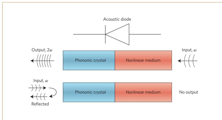
**Figure 1** | The acoustic diode. The diode consists of two segments. The phononic crystal is a periodic array of water and glass layers. The nonlinear medium is a layer of ultrasound contrast agent microbubble suspension.
